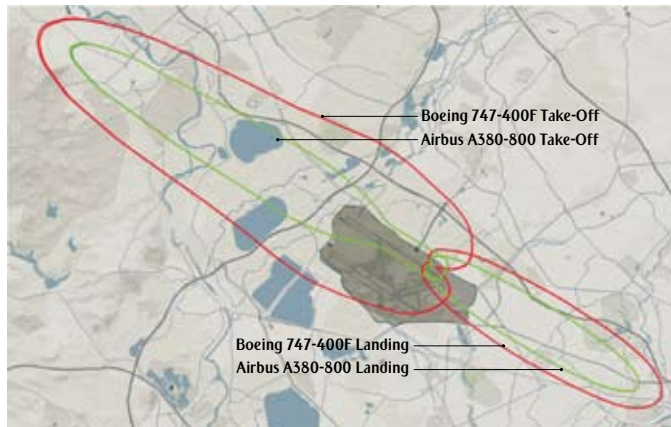
Noise Contour Map Showing Take-Off and Landing Noise Footprints of Airbus A380-800 Compared to Boeing 747-400F Aircraft
